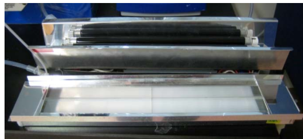
Figure 25 Flow Reactor with Removed Cover
